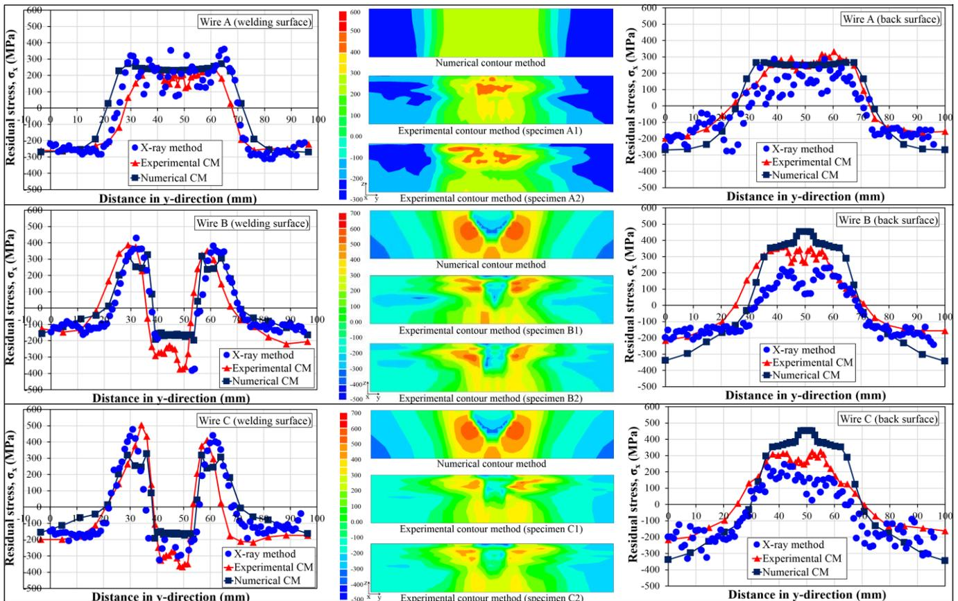
Fig. 3 Validation of residual stresses for the three weld wires with the 2D cross-sectional stress maps.
