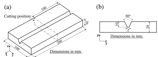
Fig. 1 Schematic drawing of test specimen. (a) test specimen geometry and (b) joint geometry.
