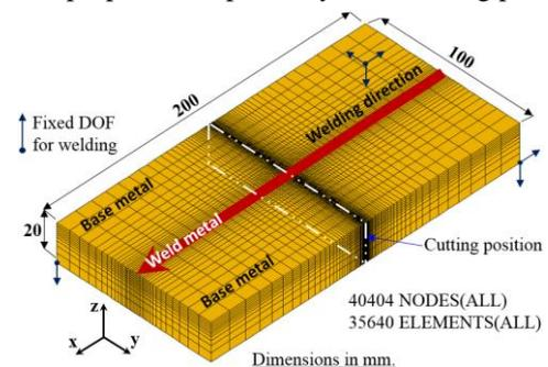
Fig. 2 FE model with locations of welding line and cutting.
